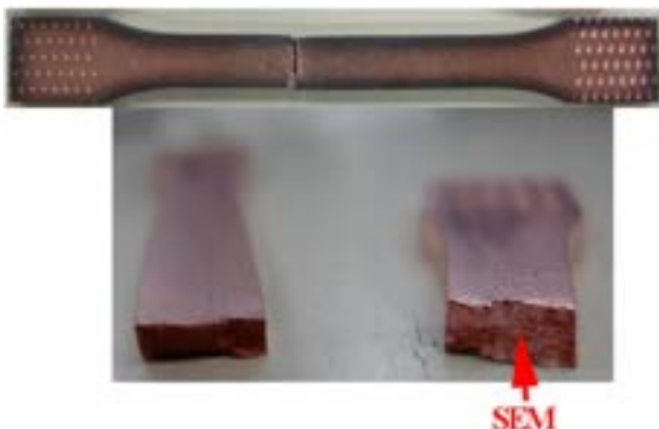
Fig. 7. Observation location of the fractured specimens.
