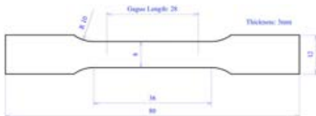
Fig. 3. Dimensions of tensile specimen.
